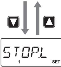
Select an option to determine pump behaviour with STOP signal.
